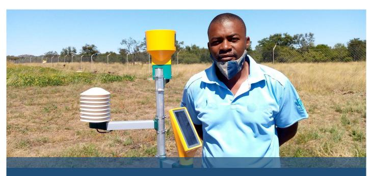
Solar powered smart weather stations at the ACEs to provide weather forecasts to farmers within a 40km radius of the stations. The stations automatically compile weather data and sends it to a portal where the responsible focal person can access and share with farmers. This will improve farmers' decision making for production.
